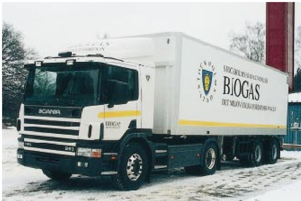
The growing interest in the use of vehicles powered by gaseous fuels. Scania built its first biogas-powered truck for the City of Stockholm.
