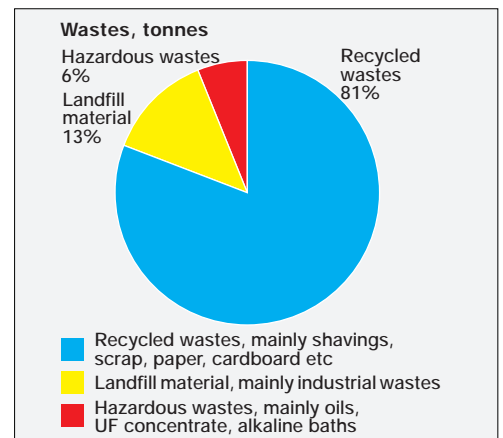
The quantity of wastes in 1997 totalled 59,000 tonnes. More than 80 percent of wastes mainly shavings and scrap, is recycled.
